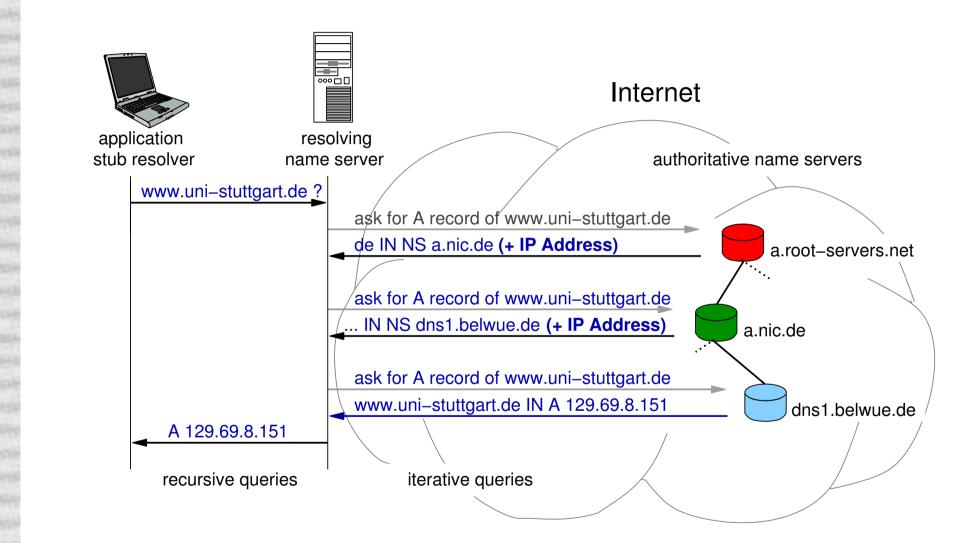
Query algorithm in Resolver – simpler clients & caching possible
