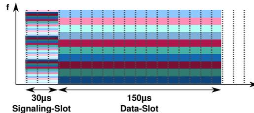
Figure 2. OFDM frequency time diagram with Codeblocks
