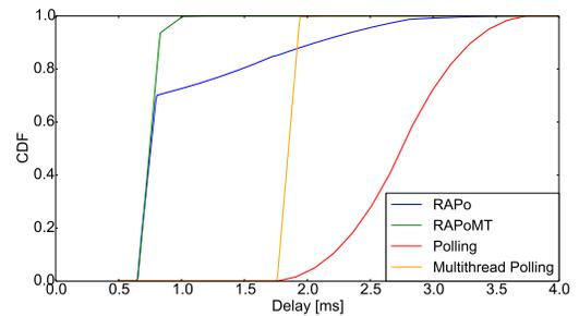
Figure 8. CDF of the delay, 40% offered load
