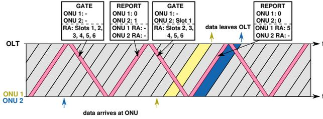
Figure 5. Principle of the combination of RA and CA
