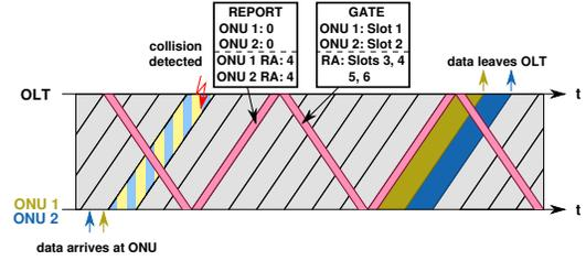
Figure 6. Reaction to collisions
