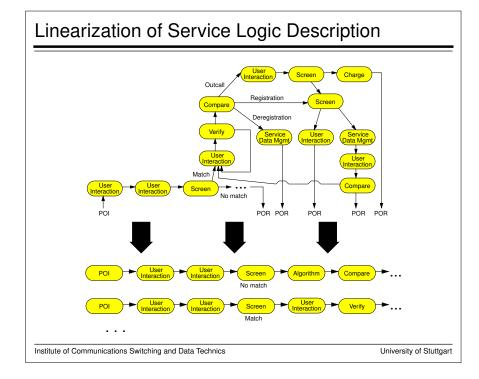
The basic components of IN service definitions are the SIBs. A SIB can result in distinct information flows in the physical plane. The information which SIB is executed is usually not sufficient. A SIB can result in very different information flows depending on several factors. Therefore a more detailed view of the SIBs must be taken into consideration.
