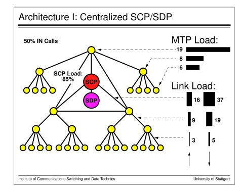
We introduce a UPT-like service with mobility management. All local exchanges can act as Service Switching Points. We add a centralized SCP which is connected via a high speed link to an SDP.
