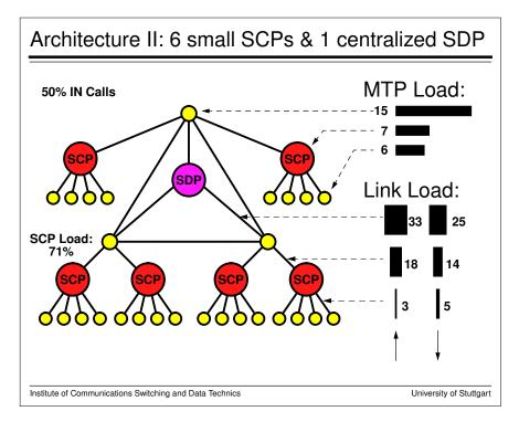
An alternative architecture is composed of six small SCPs (a fifth of the size of the centralized SCP) which are placed closer to the SSPs. We still keep a centralized SDP which stores user data like authentication keys and location information.
