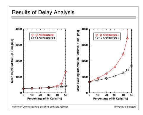
Although the load analysis did not show a fundamental difference between the two network architectures, the delay analysis does show some differences. The two figures illustrate the impact of the introduction of the new IN service on the call set-up time of ordinary ISDN calls and on the routing information retrieval time for incoming calls to subscribers of the UPT-like service. The percentage of IN calls (or subscribers) varies from 0% to 50%.
