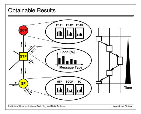
The results of the analysis include service- and protocol-specific loading of network entities like signalling links, signalling protocol processors and IN physical entities, delay of specific messages in the signalling network and in IN nodes, and service-specific grade of service criteria like e.g. mean post-selection delay.
