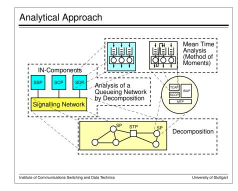
The Performance analysis is conducted using hierarchical decomposition techniques, allowing a detailed consideration of the applied protocols and the (vendor- specific) implementation of physical entities in the network.
