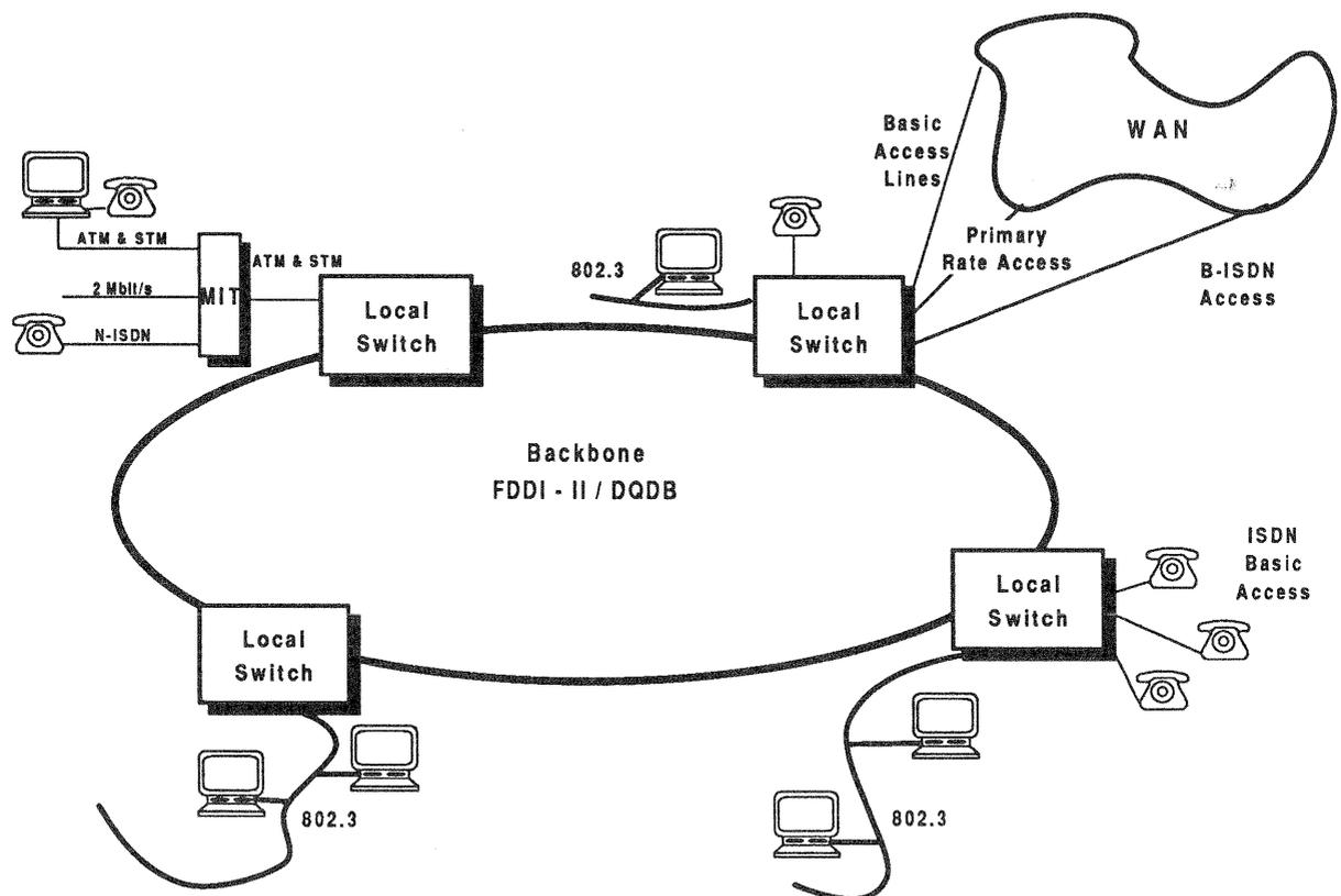
Figure 2: Architecture of a Distributed ISPBX System
