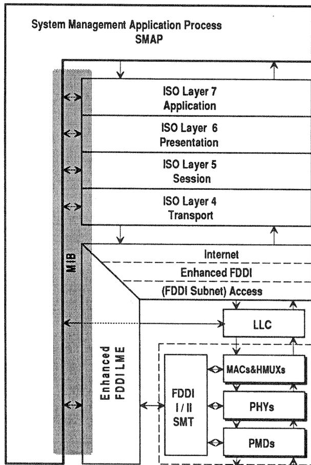
Figure 6: Layered Structure of the enhanced FDDI Station
