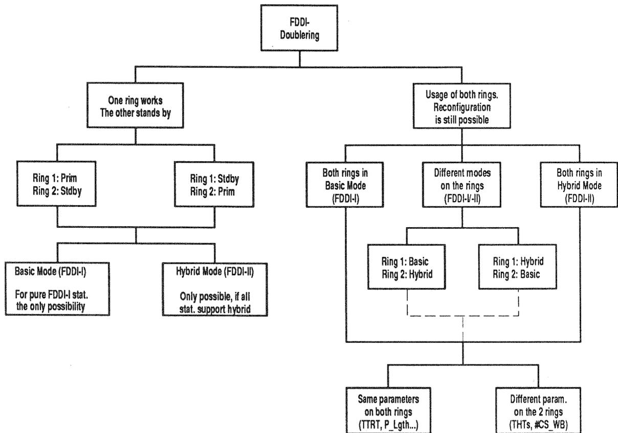
Figure 3: Possible modes on an FDDI dual ring network
