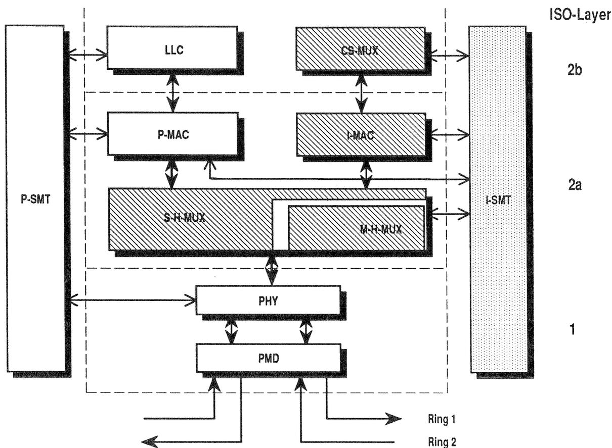
Figure 2: Block Diagram of FDDI-II Stations
