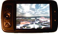
**Figure 1: High-quality rendering of a 3D city model on an O2 XDA Flame. The textured model has 23k polygons and renders at 5 frames per second.**
