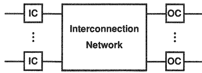
Figure 1. General model of an ATD switching element
