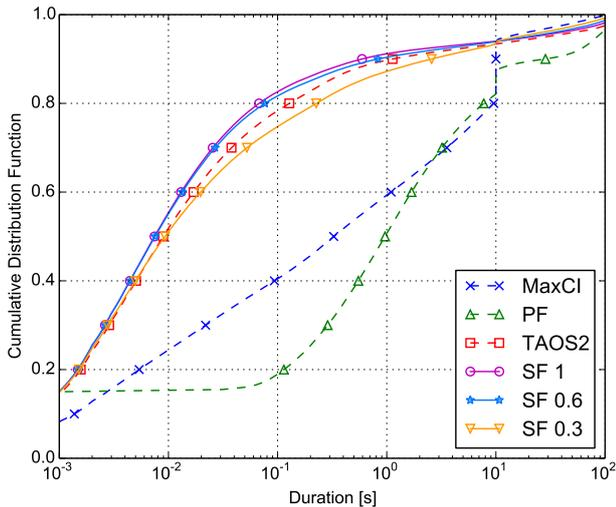
Figure 4. Cumulative distribution function of transaction durations (40 Mbit/s offered traffic).
