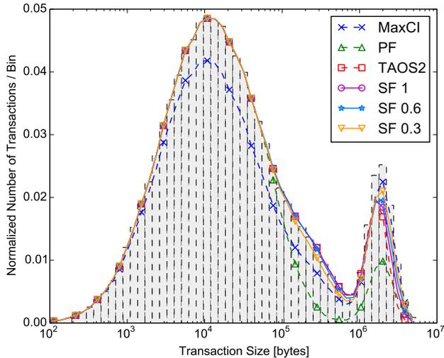
Figure 5. Histogram of finished transactions over size on a logarithmic scale (40 Mbit/s offered traffic).
