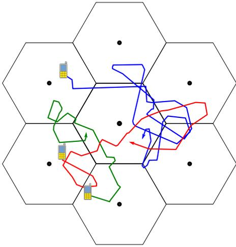
Figure 1. Cellular network layout; 7 sites with moving users and wrap-around.
