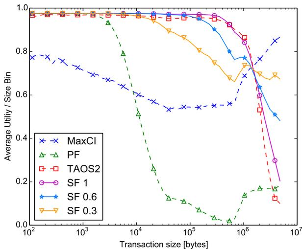
Figure 6. Average utility per bin of the logarithmic size histogram in Fig. 5 (40 Mbit/s offered traffic).
