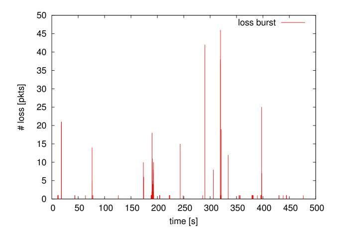
→ Irregular but few, small burst losses and very few large burst losses (as traffic model does not reflect web-browsing accurately)
