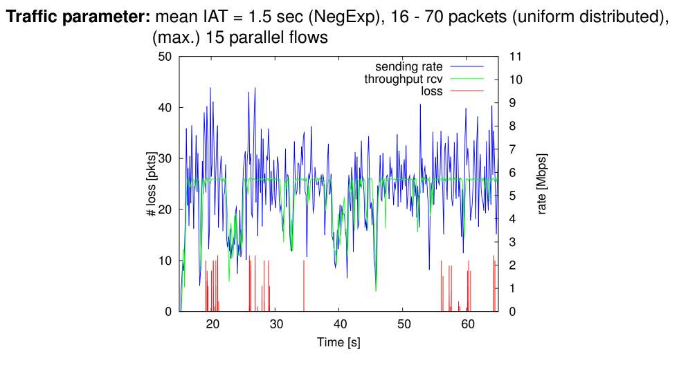
→ Smaller, random loss bursts depending on network load and flow size (1 - 11 packets in periods of full load)
