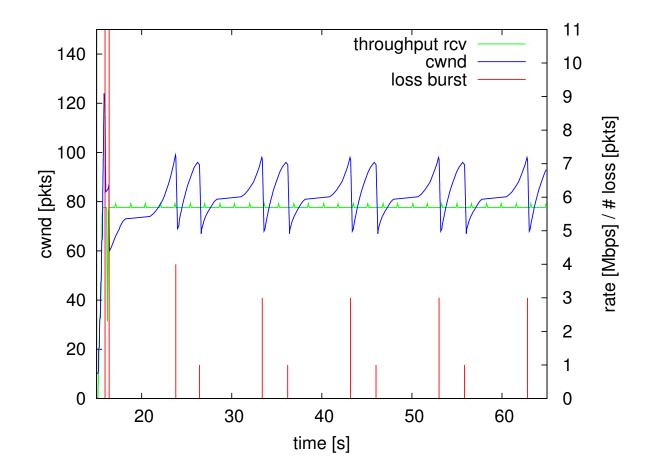
→ Regular loss pattern with periodic loss distance (1 or 3 packets per burst loss and a loss distance of 2.82 sec or 6.98 sec)
