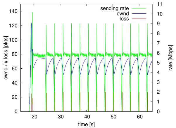
→ Regular large burst loss at the beginning of each burst data transmission (27 packets every 3.2 seconds (=IAT))
