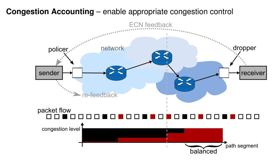
DropperDetection of permanent negative flowsPolicerLimitation of congestion volume (pos. marked packets, Token-Bucket principle)Inter-Domain Policer (Border-charging, flow control, routing)
