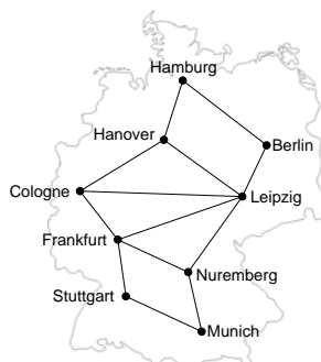
Fig. 2: Germany Network Scenario total traffic = 1 Tbps (large: 4 Tbps), mean number of \lambda s/link = 5.43 (large: 27.15)
