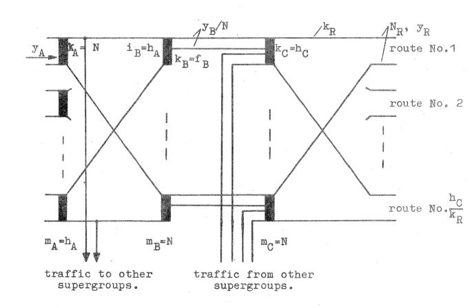
Fig. 4 Three Stage SDM Link System
