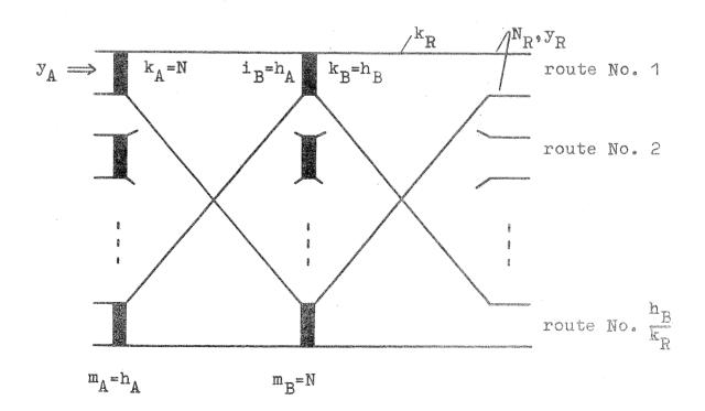
Fig. 2 Two Stage SDM Link System
