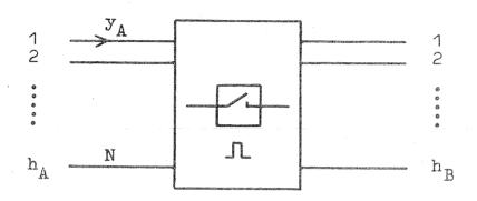
Fig. 1 Two Link TDM Switching System
