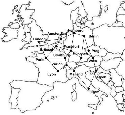
Fig. 3. Pan-European Network Scenario, total traffic=1 Tbps, mean number of \lambda s/link=5.43
