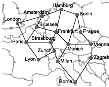
Fig. 11. COST 266 reference network with 16 nodes.
