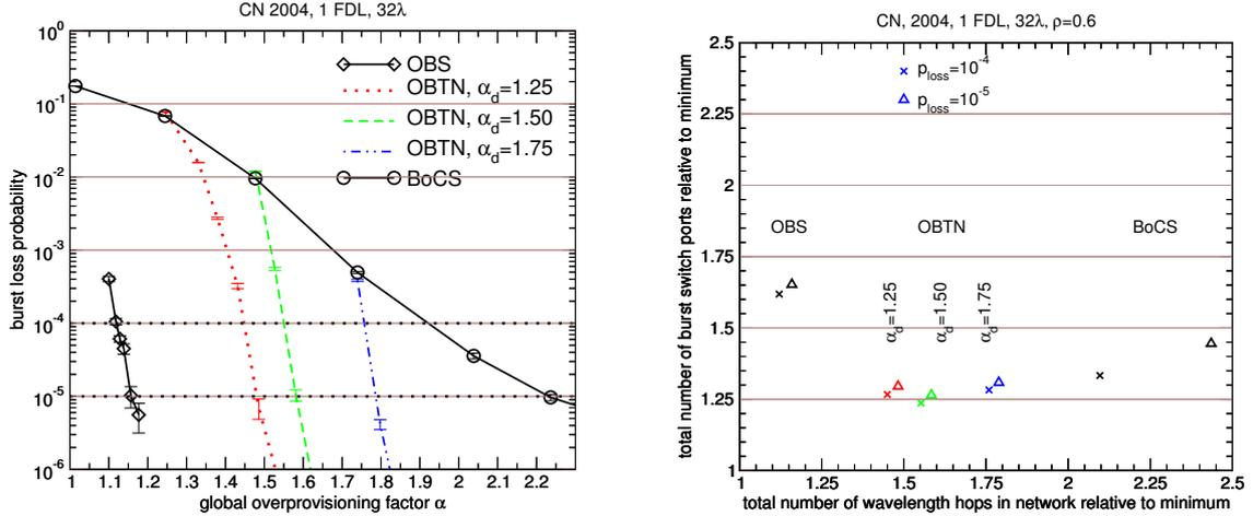
**Figure 4.** Effect of overprovisioning factor and share of overflow capacity on burst-loss probability (left); integrated architecture comparison of node complexity and network efficiency for two QoS values (right)
