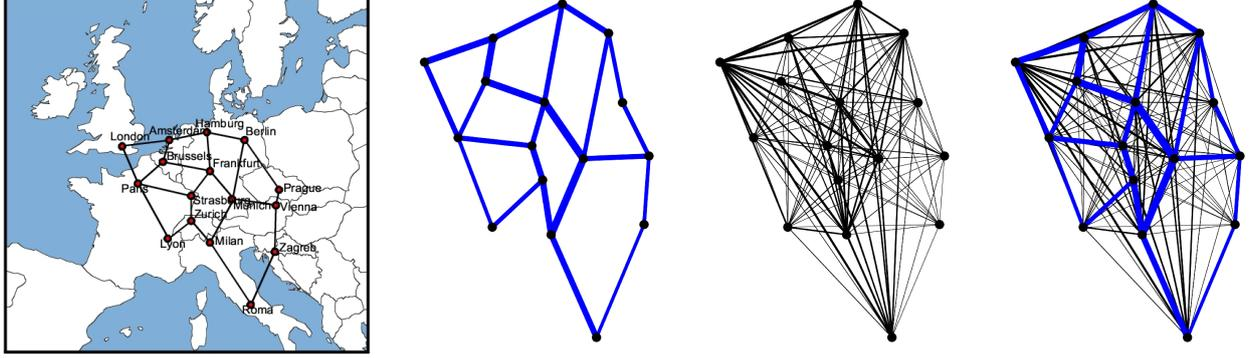
**Figure 3.** Burst layer topologies: (a) European reference network topology (b) OBS virtual topology (c) BoCS virtual topology, and (d) OBTN virtual topology (line width not drawn to scale).
