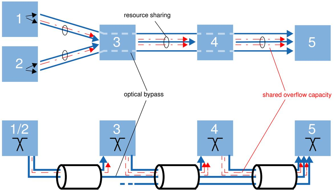
**Figure 2.** Example OBTN network segment with 5 nodes for OBTN with traffic demands  $A_{1,3}, A_{2,3}, A_{1,5}, A_{2,5}, A_{3,4}, A_{4,5}$
