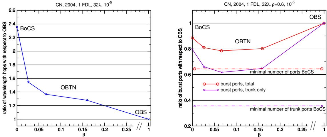
**Figure 5.** Comparison of node and network resources for OBS ( $\beta = 1$ ), BoCS ( $\beta = 0$ ), and OBTN( $0 < \beta < 1$ )
