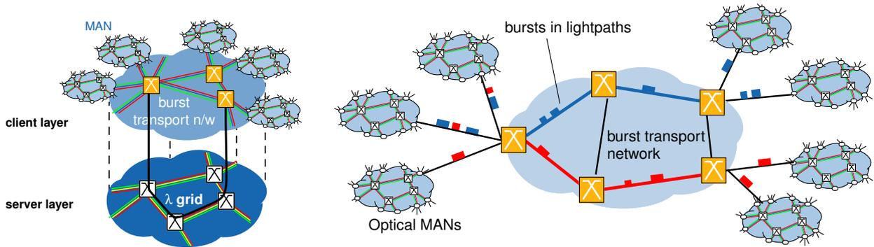
**Figure 1.** Transport network scenario: (a) burst transport and a wavelength-routed network layers and (b) interconnection of burst-switched optical MANs using lightpaths
