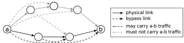
Fig. 1. Illustration of routing options along fixed path in the physical topology
