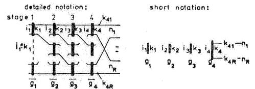
Fig. 6. Notations for 4-stage link systems without linkblocks.
