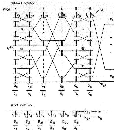
Fig. 7. Notations for 6-stage link systems.
