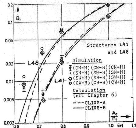
Fig. 16. Wiring and hunting in 4-stage link systems (here  $A_r/n_r = A_{tot}/N_{out}$ ).
