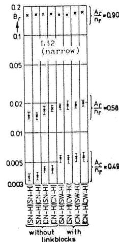
Fig. 14. Wiring and hunting in a narrow 3-stage meshed link system (here  $A_r/n_r = A_{tot}/N_{out}$ ).
