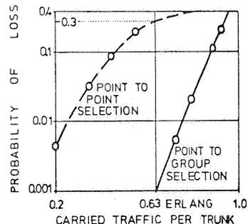
Fig. 1. Probability of loss versus carried traffic per trunk in case of point-to-point selection and point-to-group selection (simulation results for structure L42, Fig. 9).
