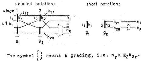
Fig. 2. Notations for 2-stage link systems.
