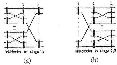
Fig. 4. Linkblocks in 3-stage link systems.
