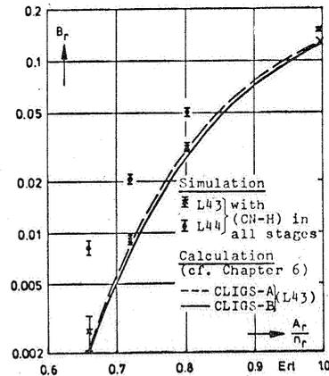
Fig. 24. The influence of  $i_1 = k_1$  in a 4-stage link system (here  $A_r/n_r = A_{tot}/N_{out}$ ).
