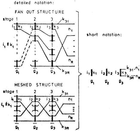
Fig. 3. Notations for 3-stage link systems.
