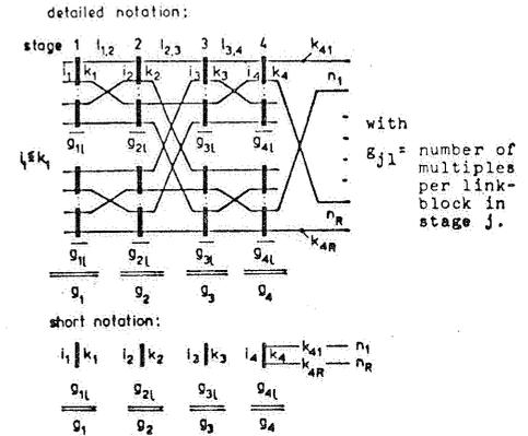
Fig. 5. Notations for 4-stage link systems with linkblocks.
