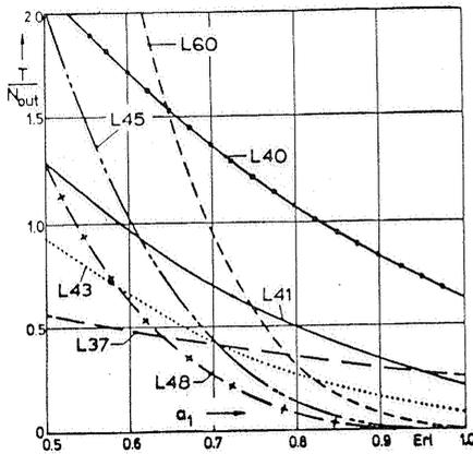
Fig. 22. Transparency of link systems having about 8000 cross-points each.
