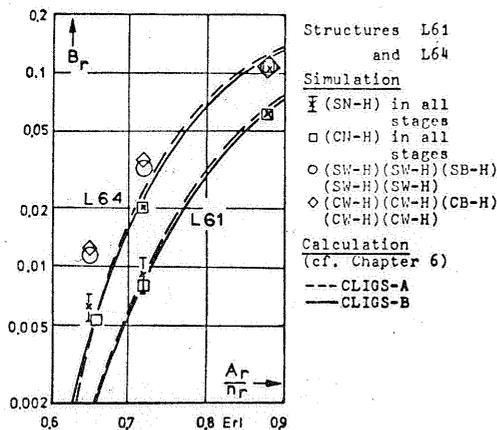
Fig. 18. Wiring and hunting in 6-stage link systems (here  $A_r/n_r = A_{tot}/N_{out}$ ).
