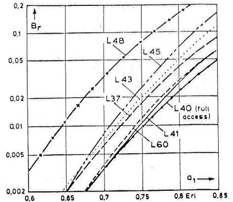
Fig. 21. Loss in link systems with about 8000 crosspoints (simulation results only).
