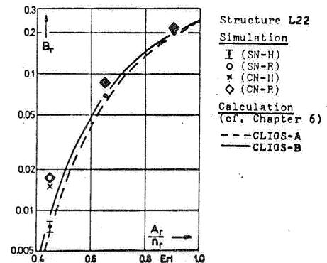
Fig. 12. Advantage of (SN-H) in case of graded trunk groups (here  $A_r/n_r = A_{tot}/N_{out}$ ).
