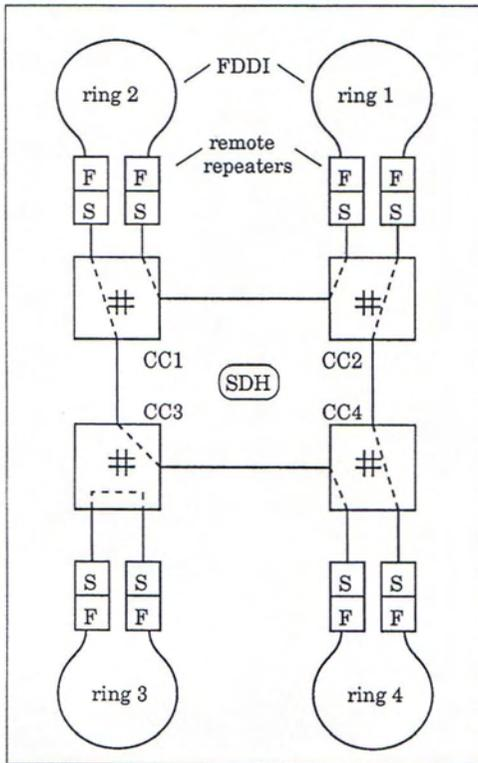
Fig. 9: Flexible Interconnection via SDH Cross Connects (CC)
