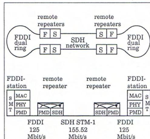
Fig. 1: Topology and Protocol-Structure of an Interconnection at the Physical Layer via Remote Repeaters
