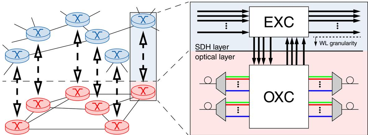
**Fig. 1** SDH-over-WDM multilayer network and node
