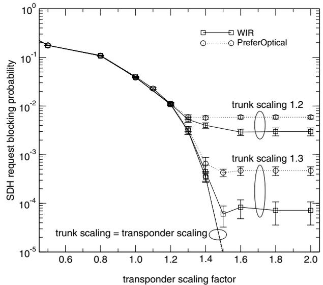
**Fig. 3** Scaled transponder dimensioning
