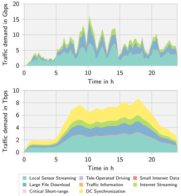
Fig. 3. Top: Highly volatile traffic demand of automotive mobile objects in one example region of the network (stacked). Bottom: Total traffic demand over time of automotive mobile objects with the edge cloud approach within the whole BB-area (stacked).
