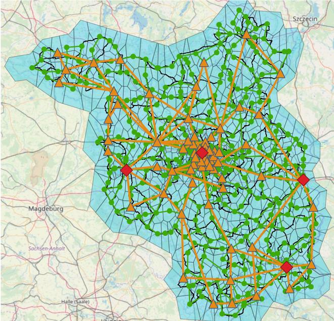
Fig. 2. BB-area fiber cable and *future* reference network: fiber cable paths in black, CO-rings in green, metro-rings in orange. Regional clustering for automotive traffic in blue, one region per node, background from [2].
