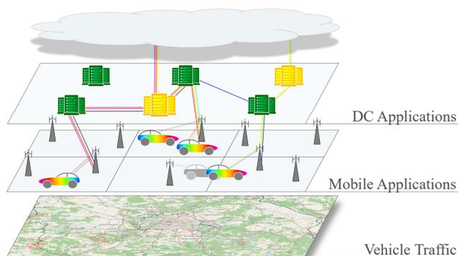
Fig. 1. The different domains to be modeled in this scenario: vehicle traffic, future automotive applications, transport network and DC applications.
