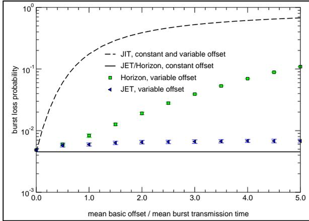
Fig. 4. Dependence of the burst loss probability on the offset
