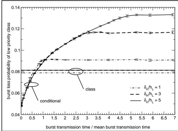
Fig. 7. Low priority losses against burst length for  $n = 4$
