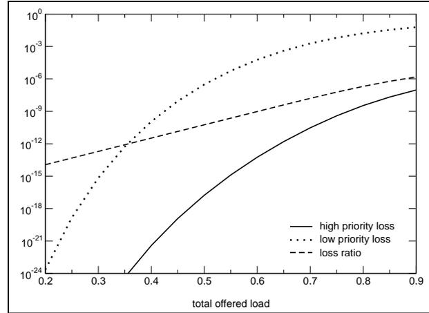
Fig. 8. Burst loss probability against load ( $\delta_H/h_L = 1, n = 64$ )
