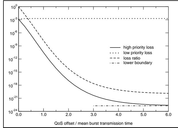
Fig. 6. Burst loss probability for 64 wavelengths and load 0.7
